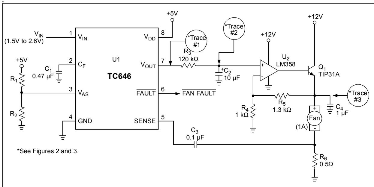
**FIGURE 1:** Linear Voltage Speed Control Circuit.
