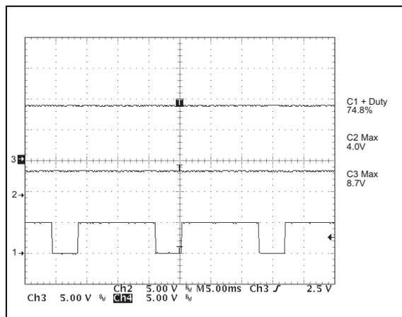
**FIGURE 3:** Waveform at 75% Duty Cycle.
