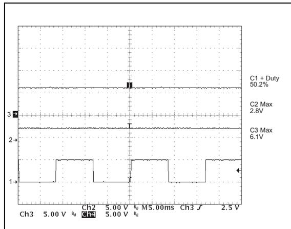
**FIGURE 2:** Waveform at 50% Duty Cycle.
